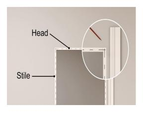
Place a length of architrave along the face of the door frame and using your pencil, mark the architrave were the two margin marks meet. This mark will indicate were the architrave will be mitred at 45 degrees. Ensure the mitre saw cut is made within the waste side of the mark.
